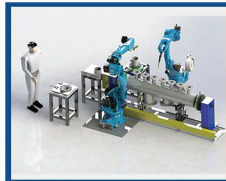
Handling and welding combine workstation-1
