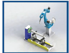
Welding robot with single-axis roller positioner
