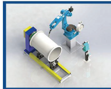
Welding robot with roller positioner
