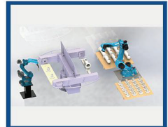
Handling and welding combine workstation-2
