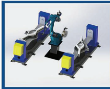
Welding robot with 2 sets of positioners equipped with clamps
