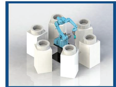
Welding robot with multiple workstations
