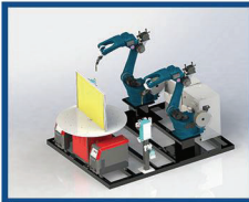
Double welding robots with single-axis horizontal positioner
