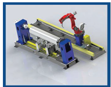
Welding robot with track & roller positioner
