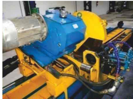
NC Flying Cold Saw Cut Off System
