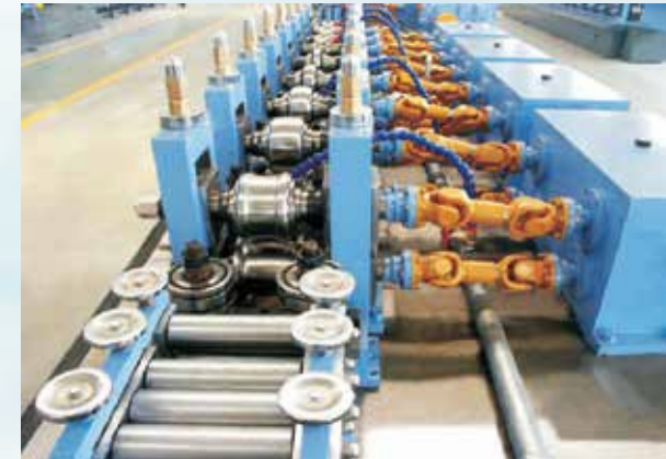
89mm ERW Pipe Mill
