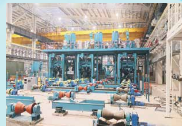
Pre Welding And Precision Welding Pipe Mill
