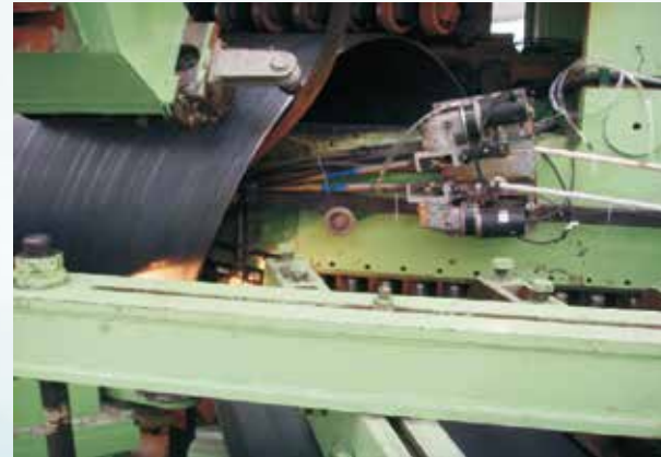
Internal Welding Machine
