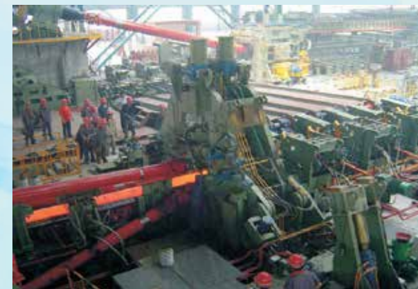
Assel Rolling Mill
